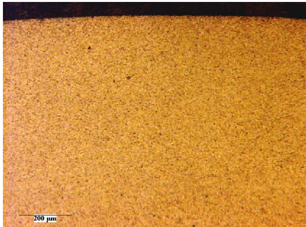
Fig. 4. Optical photograph of the steel surface during 15 min treatment.
